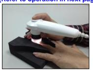
Method 2: Easy stand operation You can also fix the handy probe on a stand, adjust the working distance to get right focus & clear image.
