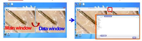
(3) If you will continue capturing images, press "Frame Freeze" button to release the frozen image (make Main window live), press again to freeze new image and press again to move it the right Data window. Then you can save this new frozen image.
